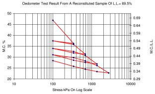
The virgin compression line can be clearly seen with the branching unloading and reloading lines. This is not representative of its undisturbed natural state but it does show the general signature of the consolidation process.
